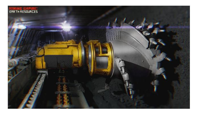
The shearer is a combined mining machine that mechanizes technological operations in the longwall, separating the mineral from the reservoir mass and loading it onto a transport machine.
